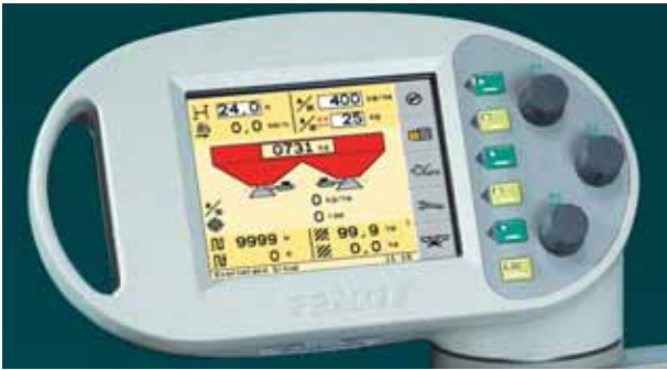
Data from implements with ISO-BUS capability is recorded automatically.
