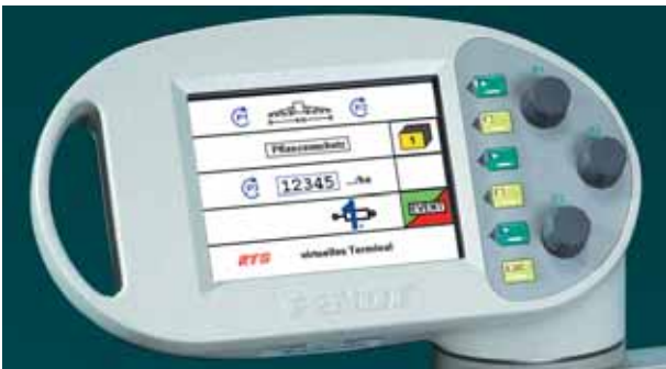
Using the "virtual ISO-BUS implement", implements that do not meet the ISO-Bus standard can use all MoDaSys functions.
